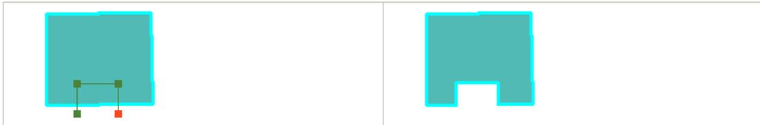
**Tip:** If you want to reshape a feature to match another one, you can use the Reshape Feature tool in conjunction with the Trace construction method. Select the feature, click the **Reshape Feature** button, click **Trace** from the palette on the *Editor* toolbar, then follow along the edge to the reshape feature.
